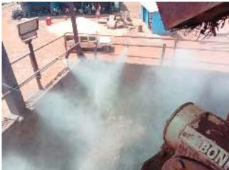
Photo #2 Showing Drilling Machine with Water Injecting System & dust suppression on the mineral transport route
